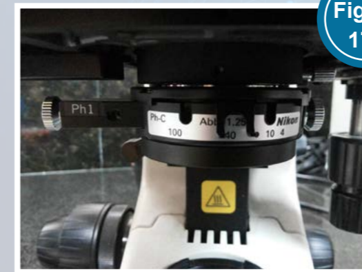
Figure 17a: A phase-contrast microscope is recommended for assessing a semen sample.
