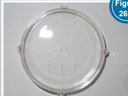
Figure 26a: PICSI® Dish that binds mature sperm with high Hyaluronon binding ability. (Cat.No BCT-PICSI-20 20 PICSI® Dish, Manufactured by Biocoat, Inc, Distributed by ORIGIO a/s Knardrupvej 2, 2760 Måløv, Denmark
