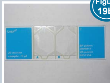
Figure 19b: Leja ® slides are high quality disposable counting chambers for semen analysis with chamber depth of 20 µm for increased level of accuracy and precision (Manufactured by Leja Luzernestraat,10 2153 GN Nieuw-Venep, The Netherlands)
