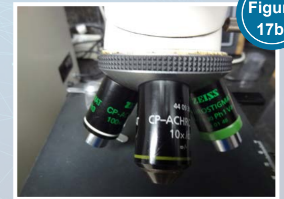
Figure 17b: Positive phase objective ×10, ×20 and ×40 attached to the phase-contrast microscope for general assessment, motility, vitality, and counting of spermatozoa and non-sperm cells.
